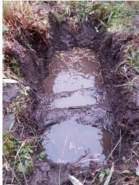
Position of water table after 2 weeks of dry weather in 16 Springfield Gardens.
